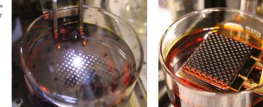
(left) A part being built up from resin and (right) coming out of the bath.
