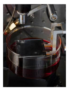
Normal projection lithography projects the image of the DMD onto a single area. The size of this image therefore determines the size of the build area and the size of the smallest feature producible. Parts larger than this limited area require the build area to be physically moved
