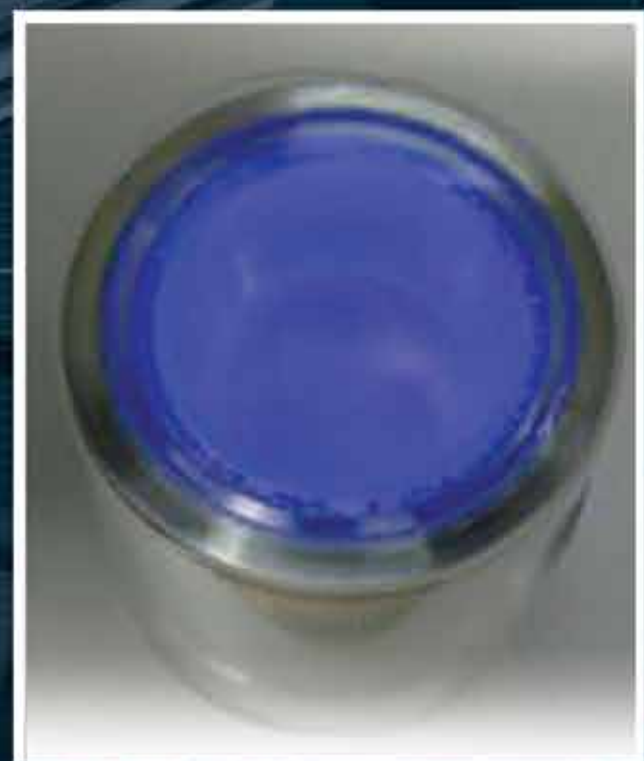
(top left) A crystal of strontium iodide doped with europium for gamma-ray detection is an R&D 100 Award winner. (top right) The crystal is encapsulated when used in a radiation detection device and (bottom) glows blue when exposed to ultraviolet light.
