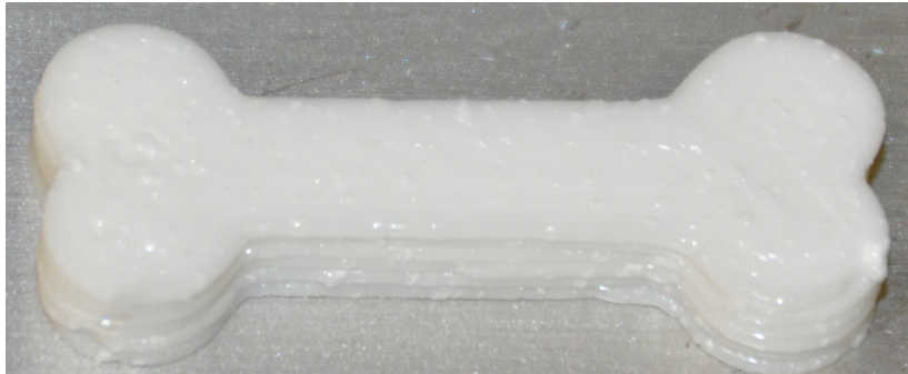
Printed AM training Aid with HMX before curing
