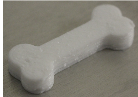
AM printed training aid with HMX uncured AM printed training aid with HMX cured
