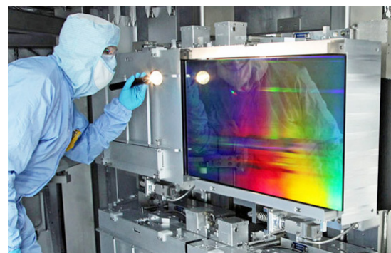
Engineer JB McLeod inspects one of the high-efficiency diffraction gratings installed at NIF. LLNL manufactures multilayer dielectric diffraction gratings up to 1 meter in diameter and optimized for a diffraction efficiency of greater than 90 percent.
