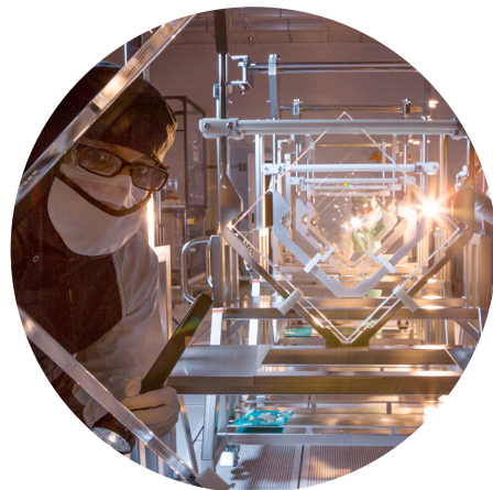
Optics Mitigation Facility operator Constantine Karkazis inspects the facility's CO 2 laser processing hardware. Credit: Bruno Van Wonerghem.
