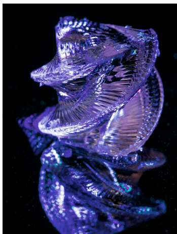
A 3D-printed helical glass structure created by LLNL engineer Du Nguyen demonstrates the capability to preserve fine features and sharp edges.
