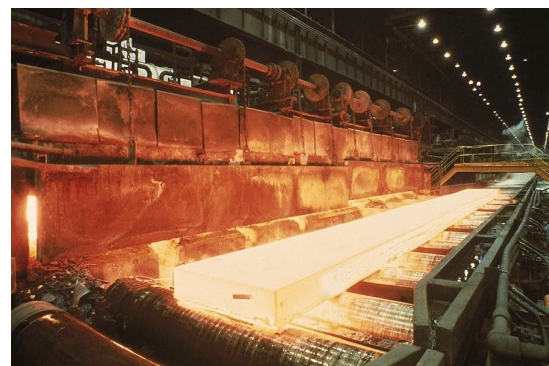
The HPC4Mfg CRADA with US Steel focuses on predicting microstructure growth during the hot strip mill process pictured above.
