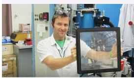
Zachary Seeley from LLNL holds a gadolinium-lutetium-oxide (GLO) transparent ceramic scintillator plate. The GLO scintillator—a technology recognized by a R&D 100 award provides imaging that is seven times faster than glass scintillators.
