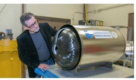
LLNL engineer Brian Guidry, one of the first recipients of an award from DOE's Technology Commercialization Fund, examines innovative cryo-compressed hydrogen tank technology.
