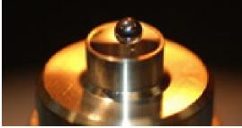
A stainless steel ball is supported by a thin sheet of plastic that is approximately 200 atoms thick, produced using the polyelectrolyte enabled liftoff (PEEL) technique. Developed by LLNL scientists Salmaan Baxamusa and Michael Stadermann, along with colleagues from General Atomics, PEEL received an R&D 100 Award in 2016, as well as a regional FLC Outstanding Technology Development award
