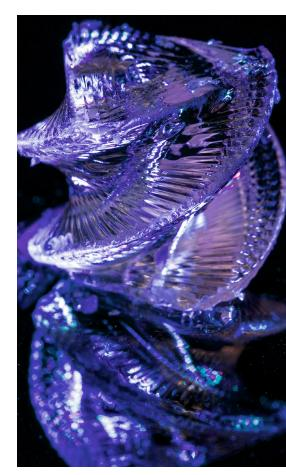
A 3D-printed helical glass structure created by LLNL engineer Du Nguyen demonstrates the capability to preserve fine features and sharp edges.
