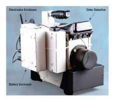
Example of how RaFTS is attached to an Ortec radiation detector, with signals injected through a port on the detector's exterior. RaFTS is detector-agnostic, enabling it to work with each trainee's specific type of detector, providing a more realistic training experience.
