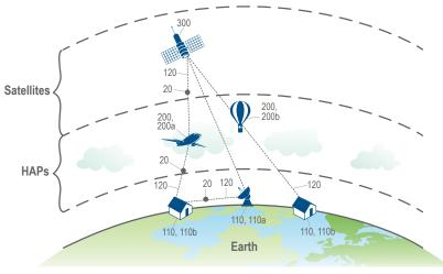
Depiction of how ground-to-satellite optical communications can travel through sensors on airplanes or balloons. (Image from Google's March 2018 patent.)
