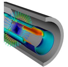
The ALE3D simulation shown depicts powerful magnetic fields generated by a large pulse of electrical current running through an outer conductor. The magnetic fields crush a thin-walled metal cylinder located inside the larger conductor. The inner cylinder is slotted to break the axial symmetry, making this a fully 3D problem.
