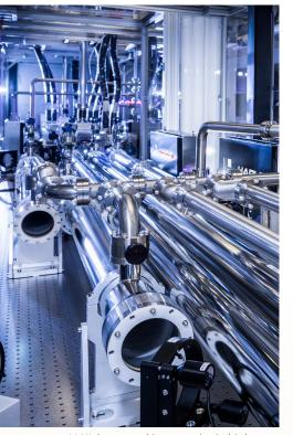
LLNL leveraged its expertise in highpower lasers through a partnership with the European scientific community to develop HAPLS, the world's first laser capable of generating 30 femtosecond pulses with peak power of more than one petawatt. HAPLS is fully integrated, operational, and is available to scientists worldwide for studying laser-matter interactions.
