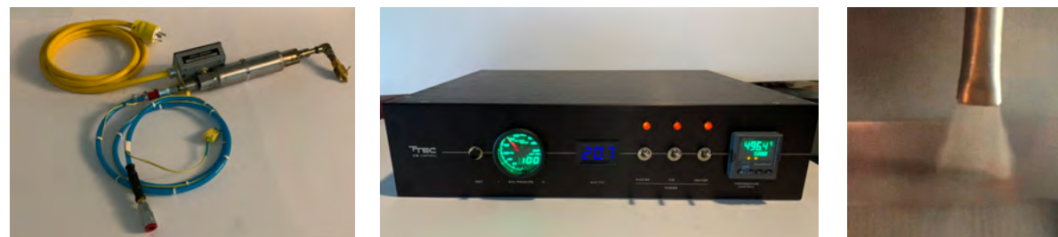
Figure 1 The streamlined VCS spray unit (left) and controller (center) are portable, enabling easy setup for coating of industrial components and materials (right).
