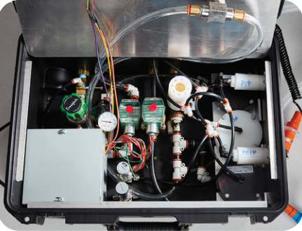
SuppleVent, a ventilator developed by LLNL and mass produced by North Carolina-based medical device startup company BioMed-Innovations is designed to help COVID-19 patients breathe.
