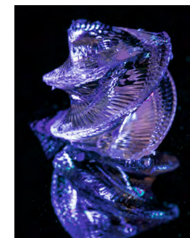
Figure 4: A 3D-printed helical glass structure created by using Tailored Glass by DIW demonstrates the capability to preserve fine features and sharp edges.
