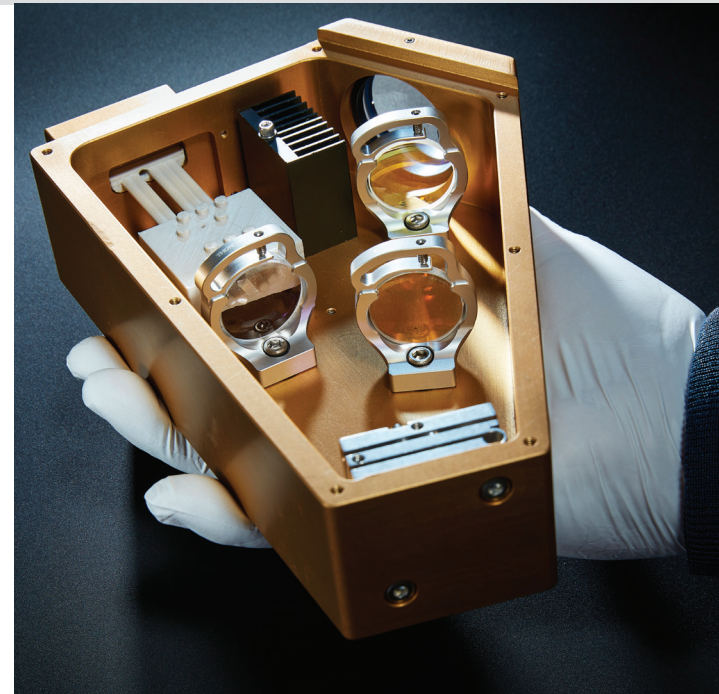
Figure 3: Prototypical EXUDE Elite SBC system capable of combining 16 input laser beams into one 48 kW output laser. It can be held in one hand, demonstrating its impressive, compact size.
